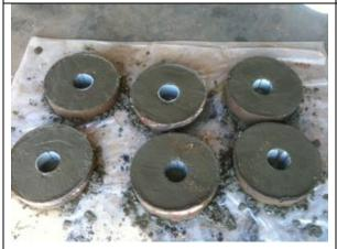
It's convenient to do several blocks at a time. 2 60-pound bags of ready-mix concrete is just right for 6 irrigation blocks.
